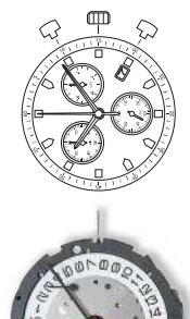
6S11 Height 4.50mm Chrono min / sec, 120 second 4 year battery life (SR927W)
