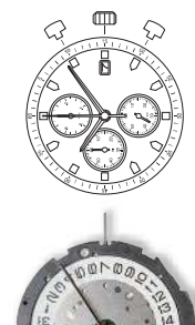
6S10 Height 4.50mm Chrono min / sec, 120 second 4 year battery life (SR927W)
