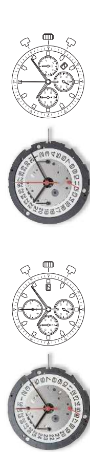
6S10 Height 4.50mm Chrono min / sec, 120 second 4 year battery life (SR927W)
