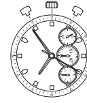
JS55 Height 4.18mm Chrono. 30min/sec. 24 hour 3 year battery life (SR621SW)
