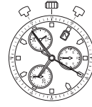
JS05 Height 4.20mm Chrono. 30min/sec. 24 hour 3 year battery life (SR621SW)
